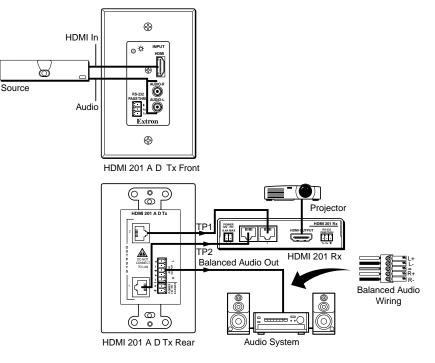
Figure 2-27 — Typical installation
